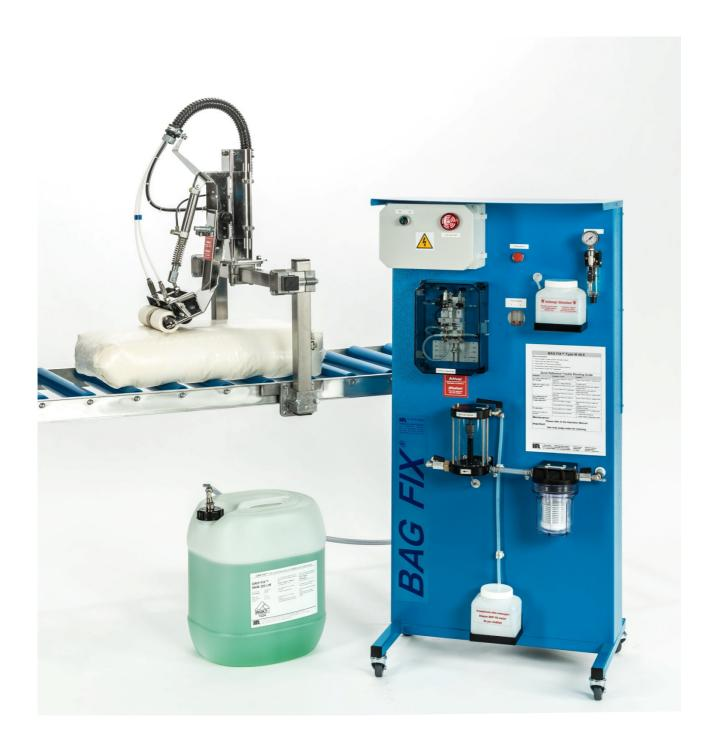
System: Sponge Roller Application with Cylinder Pumps and Disposable Container
