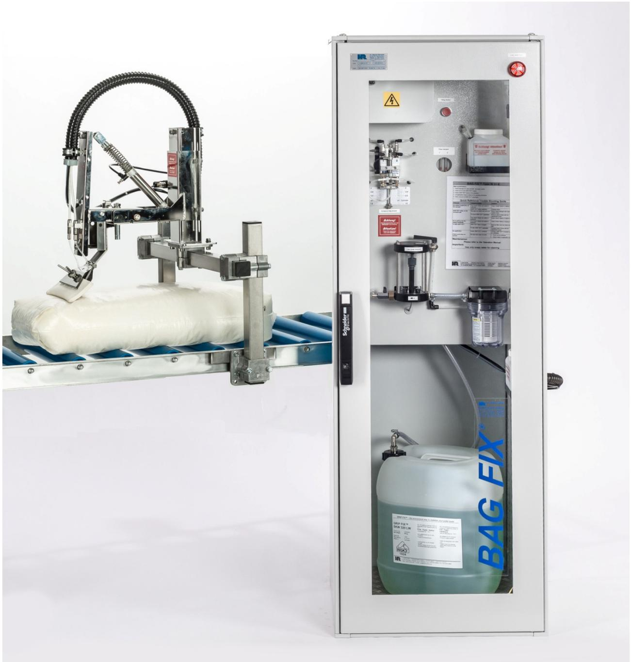
**System: Stripe Application with Cylinder Pumps and Disposable Container**
